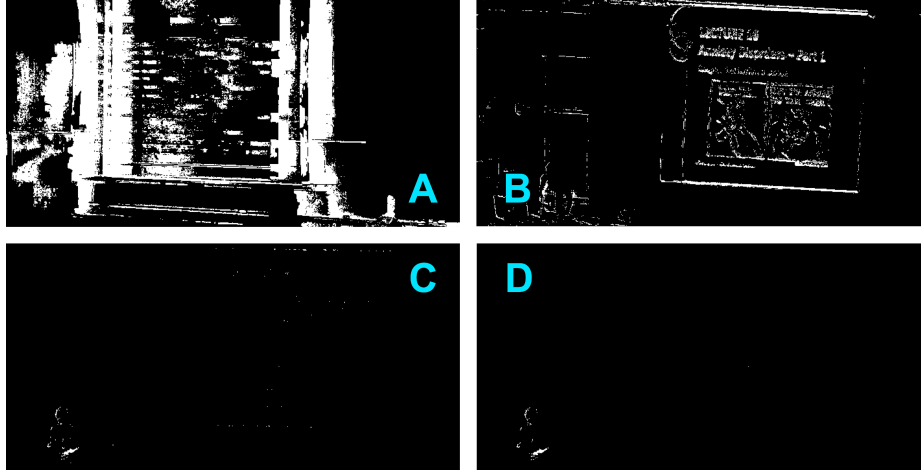
Fig. 1. Examples of three kinds of visual noise in videos: A) camera pan, B) camera vibration, and C) electronic low-light noise. Image D contains an example of smoothed motion from C with lower-left instructor motion preserved and noise visible in the upper-right of C correctly removed (zoom in for detail).
